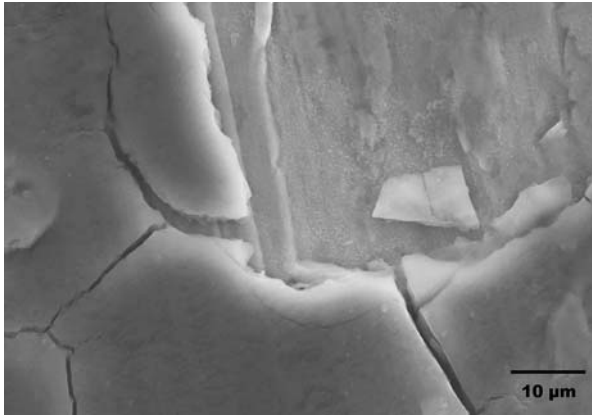
Figure 7 Brittle cracking on the wear track of untreated SS316L.
